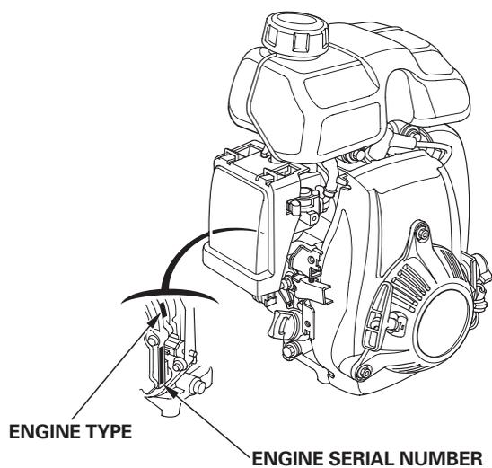
Engine serial number: \_\_\_\_\_
