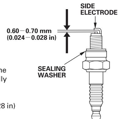
4. Measure the spark plug electrode gap with a wire-type feeler gauge. Correct the gap, if necessary, by carefully bending the side electrode. The gap should be: 0.60–0.70 mm (0.024–0.028 in)
