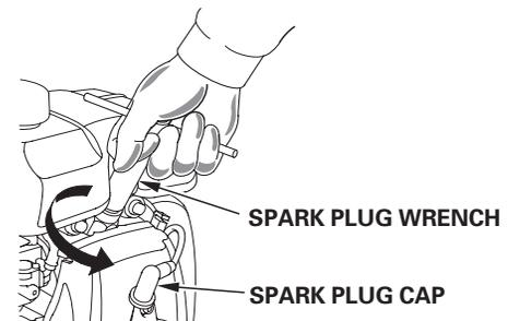
3. Inspect the spark plug. Replace it if damaged or badly fouled, if the sealing washer is in poor condition, or if the electrode is worn.
