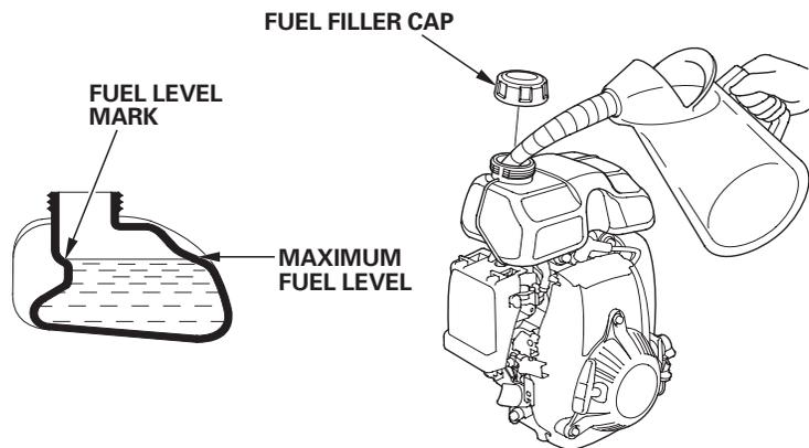
3. Refuel carefully to avoid spilling fuel. Do not fill the fuel tank completely. It may be necessary to lower the fuel level depending on operating conditions. After refueling, tighten the fuel filler cap securely.
