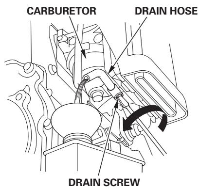
3. After all the fuel has drained into the container, reinstall the drain bolt (carburetor equipped with a drain bolt type only). Tighten the drain bolt or drain screw securely.
