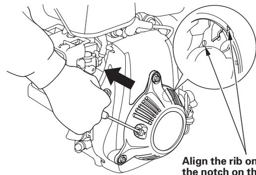
Align the rib on the flywheel with the notch on the fan cover.
