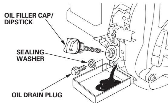
3. With the engine in a level position, fill with the recommended oil (see page 7 ) to the upper limit mark (bottom edge of the oil fill hole).
